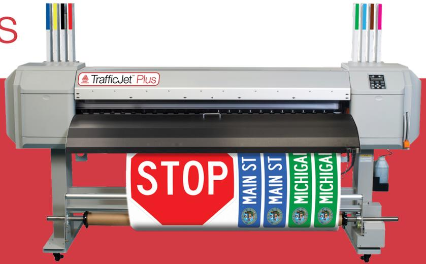
The TrafficJet Plus printer is built on a proven platform including an integrated dryer for fast print speeds up to 15 m<sup>2</sup>/hour while reducing ink consumption. CMSpot6™ inks and included software automates sign making, simplifying the printing of specification compliant traffic control, wayfinding, and custom signage.
