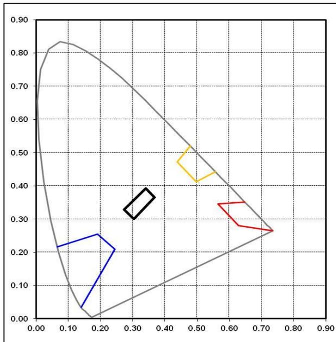
Avery Dennison HV1302 Series performance exceeds the minimum coefficients of reflection specified in Figure A and meets the ASTM D4956 Type V daytime color requirements specified in Figure B. Excluding the reflectivity and color requirements listed above, Avery Dennison HV1302 meets all performance requirements specified in ASTM D4956.
