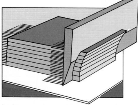
Cutting pressure should be 25 to 35 psi. If you can't adjust pressure, place a few sheets of cardboard on the lift to absorb shock. Cardboard inserts can also be used as counters. Note that these cardboard sheets are included in the 2-inch (5cm) maximum stack height.
