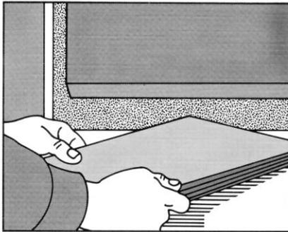
Guillotine cutting is best suited for cutting a large volume of straight edged sheets. The type and condition of the cutter will determine the accuracy, tolerances, and quality of the cut.
