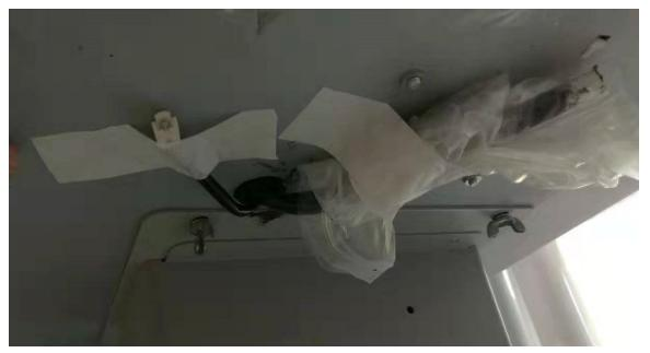
Tape both the bags securely to the underside of the printer. Place the waste tank in a large plastic bag, ensuring it is clean and empty prior to transport.
