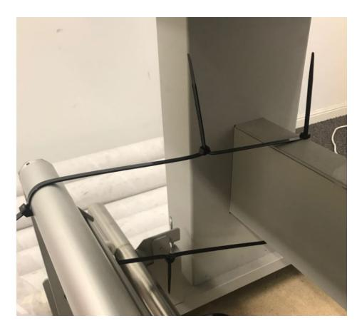
The printer is now safe to move. Brace the printer appropriately to minimize vibration and jostling during transit.
