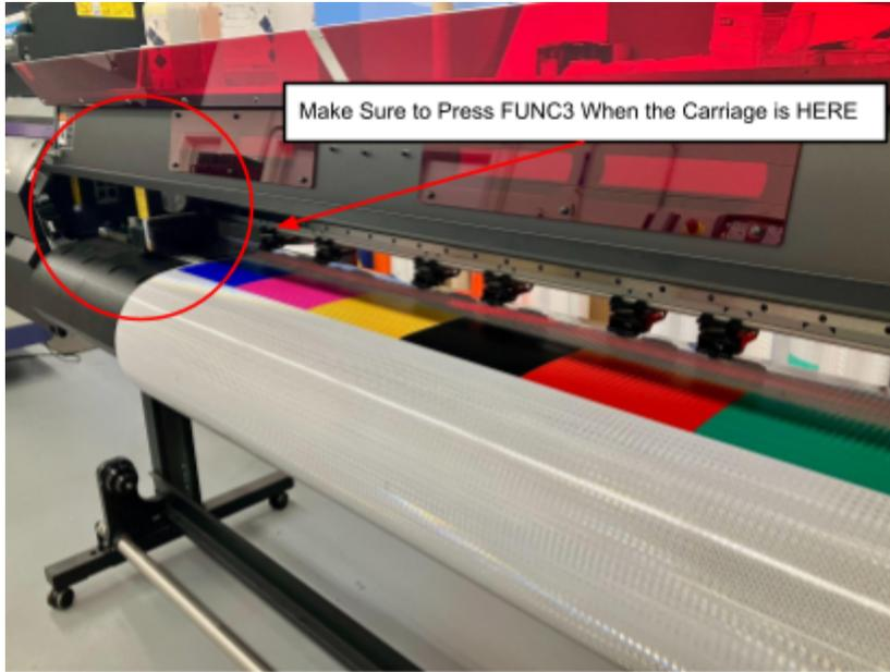
Fig 2. Printer carriage
