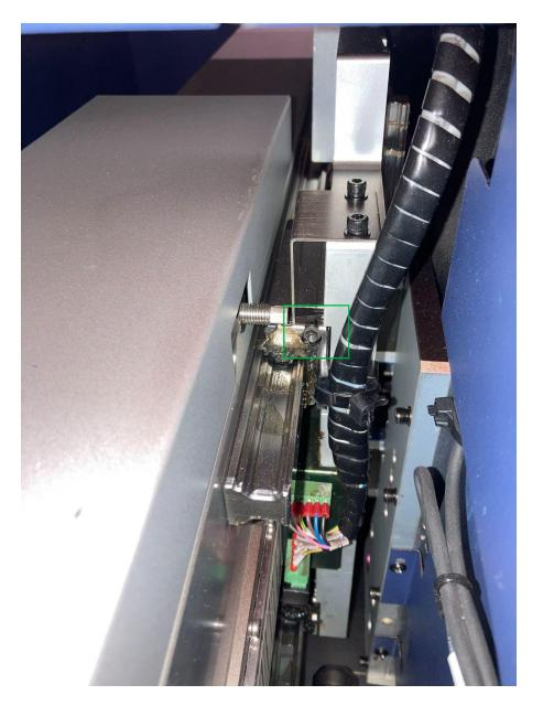
IMPORTANT: Not lubricating these parts in time, may cause catastrophic failure to the printer!
