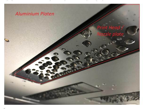
Be Careful: Do not apply excessive force on the Print heads, you may damage the nozzle plate.
