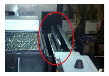
Fill the Eye Dropper (Pipette) with Flush and empty **<u>2 full</u>** Eye Droppers onto the Wiper Blade and into the bucket underneath. This will dissolve and remove dried ink in the plastic collector and tube under the Wiper Station and will help prevent clogging and ink leakage.
