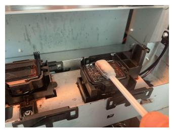
After that, fill both Cappings again with some Flush and use a dry swab to suck out the Flush from the inside of the Capping, absorbing ink buildup from the Capping filter. Continue until it looks clean.
